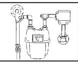
9. PROPER STABILIZATION OF THE VALVE INSTALLATION IS ESSENTIAL TO AVOID NUISANCE TRIPPING. TO STOP EXCESSIVE VIBRATION AND TO COMPLY WITH CODES. We recommend the valve is braced with Little Firefighter GV-12 Stabilizer Bracket. However, any adequate bracing system may be used.
