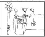
**3.** Remove the union from the house side of the meter with a pipe wrench and detach the union.
